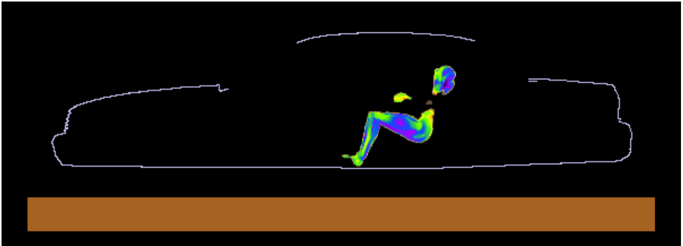
Figure 5. SAR distribution at 419.5 MHz in the passenger back center model produced by the trunk mount HAE6012A antenna. The contour plot is relative to the plane where the peak 1-g average SAR for this exposure condition occurs.
