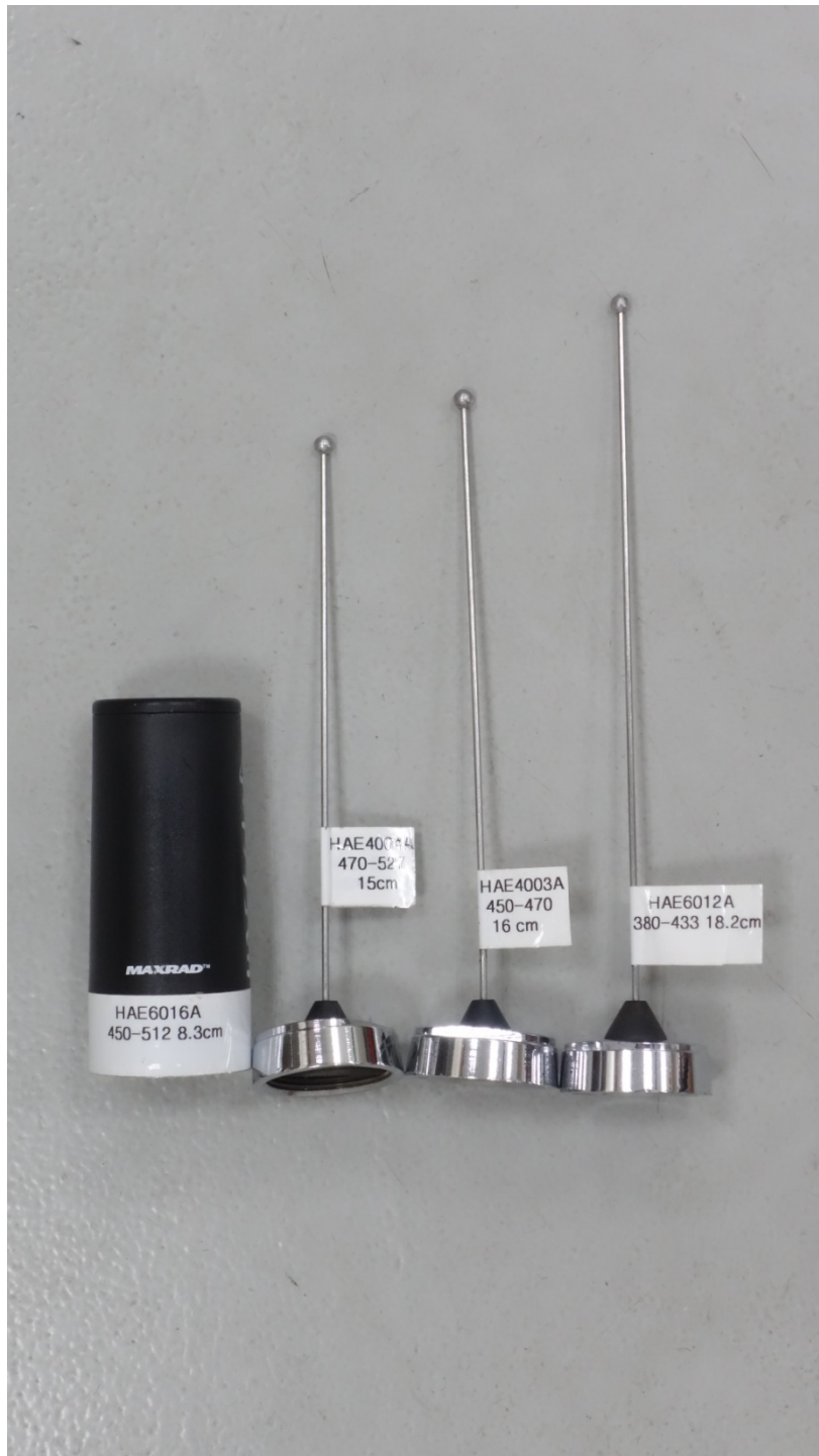
UHF Antenna kit numbers, from left to right; HAE6016A, HAE4004A, HAE4003A and HAE6012A
