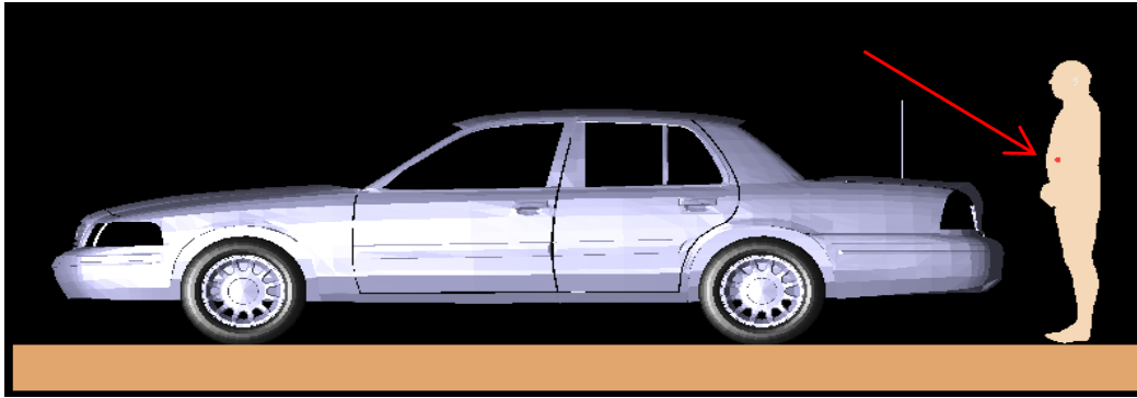
Location for the E-field sensors placed in the bystander for the convergence analysis.
