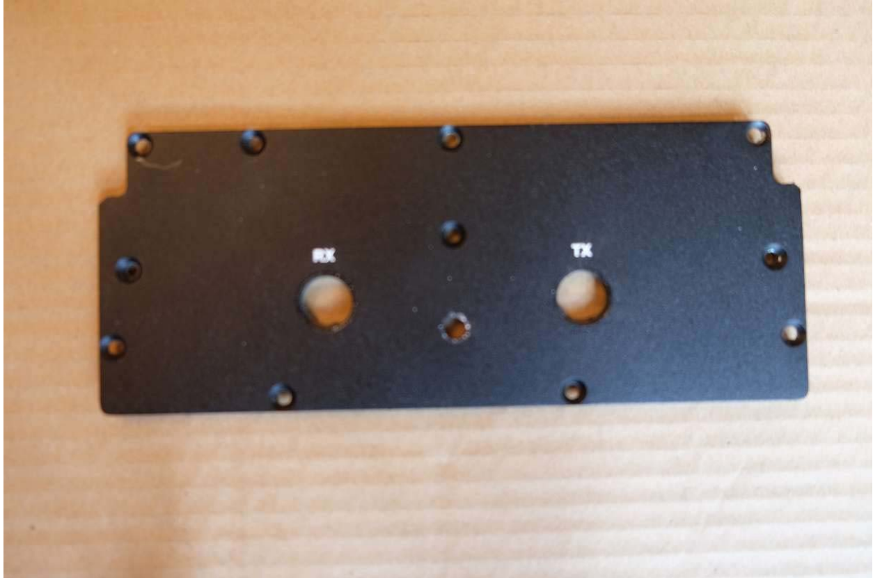
The cover is 4mm larger and the upper right screw was added
