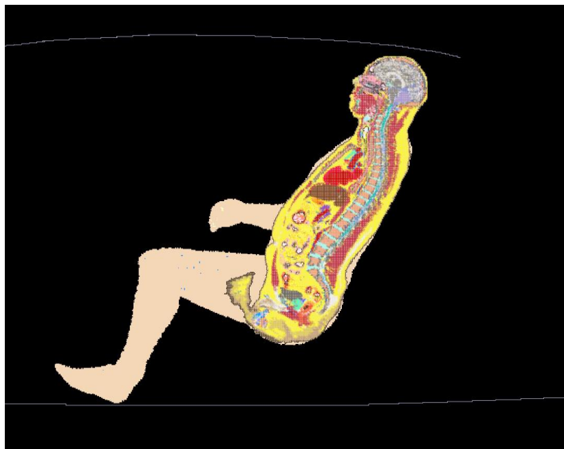
Figure 2: Passenger (back seat) model exposed to a trunk-mount antenna: XFDTD geometry. The antenna is mounted at 85 cm from the passenger located in the center of the back seat.
