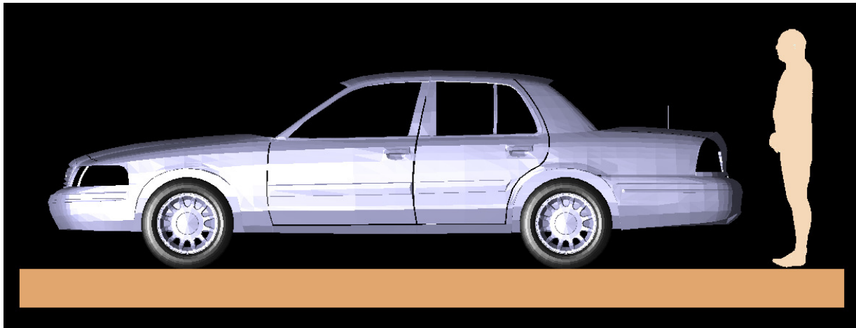
Centered bystander model at 20 cm from vehicle equipped with a trunk-mount quarter-wave monopole antenna operating at UHF (450 MHz).
