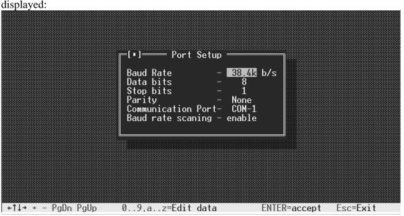
Ensure that the correct communication port is selected and set the **Baud rate** to 9600 b/s. If higher **Baud rate** is selected, ensure that the **Baud rate scanning** is set to **Enable**. Exit from the Ports menu and select "Yes" when prompted "Would you like to update config file?"
