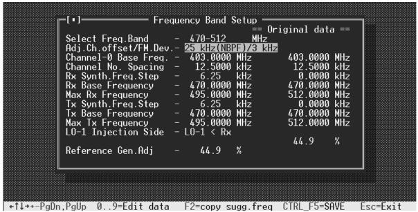
Adjust the **Adj. Ch. Offset / FM Dev** field to the correct channel spacing i.e. 25kHz (NBPF)/3kHz or 12.5kHz / 1.5kHz. All other fields must not be changed by the user.
