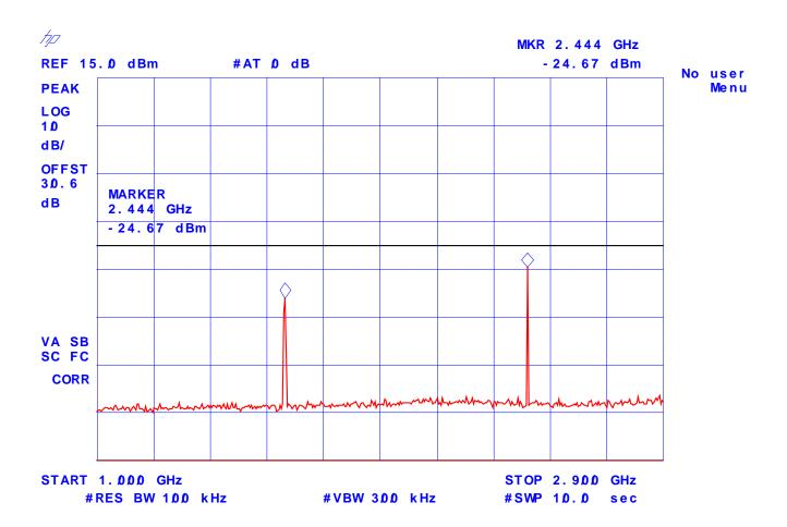
Plot # 103: Transmitter Antenna Power Conducted Emissions
