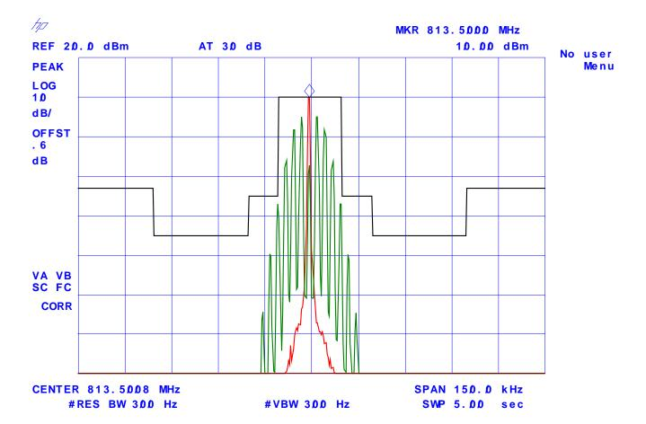
Frequency: 813.5 MHz, 25 kHz Channel Spacing. Low Power, RF Output
