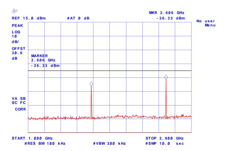
Plot # 124: Transmitter Antenna Power Conducted Emissions
