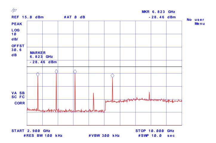
Plot # 119: Transmitter Antenna Power Conducted Emissions Frequency: 860 MHz, High Power
