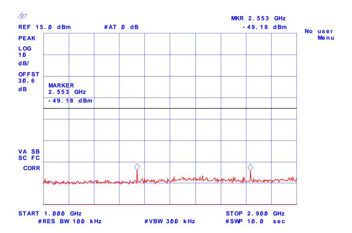
Plot # 109: Transmitter Antenna Power Conducted Emissions
