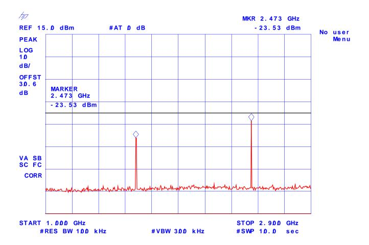
Plot # 106: Transmitter Antenna Power Conducted Emissions
