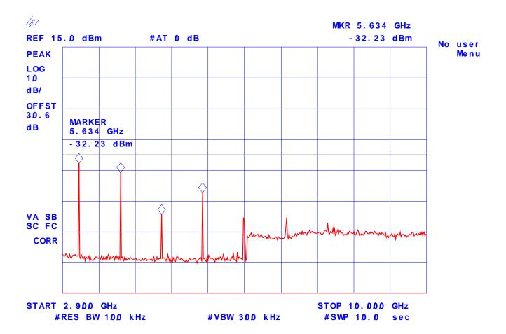
Plot # 101: Transmitter Antenna Power Conducted Emissions Frequency: 815 MHz, High Power
