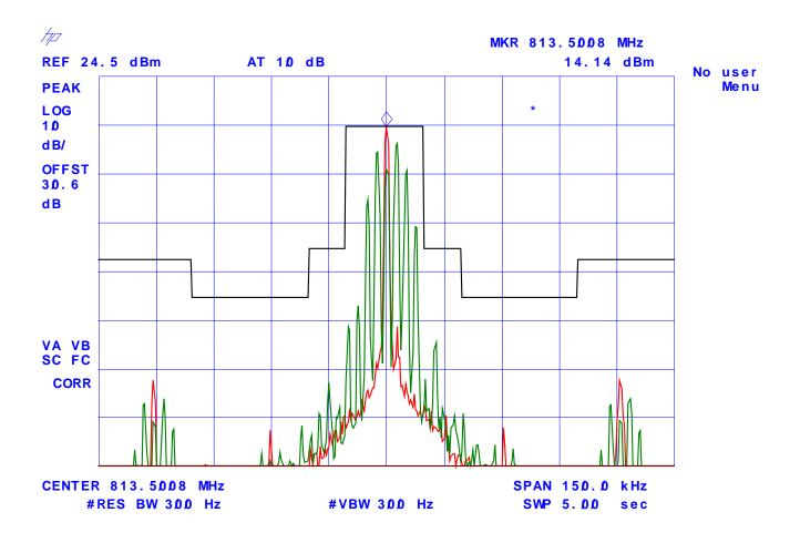
Frequency: 821 MHz, 25 kHz Channel Spacing. Low Power, RF Output
