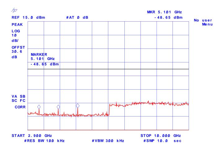
Plot # 110: Transmitter Antenna Power Conducted Emissions Frequency: 860 MHz, Low Power
