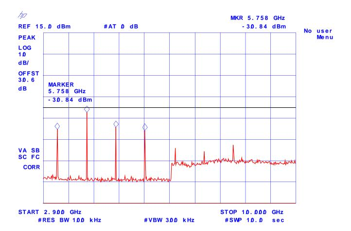
Plot # 107: Transmitter Antenna Power Conducted Emissions Frequency: 851 MHz. Low Power
