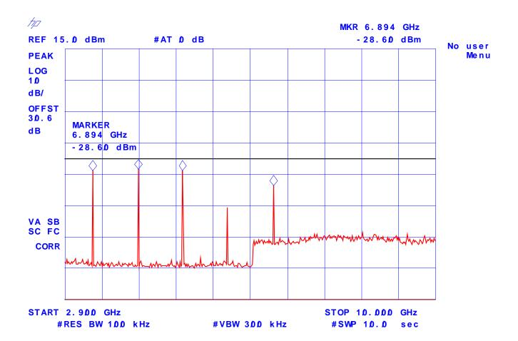
Plot # 122: Transmitter Antenna Power Conducted Emissions Frequency: 869 MHz, High Power
