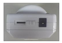
Moving the switch away from the power connector jack will put the CA9000 into either a 15-minute delay, 10-minute delay, 5-minute delay, or "pulse mode" (the pulse mode position is shown in the figure below), depending on the switch's position.
