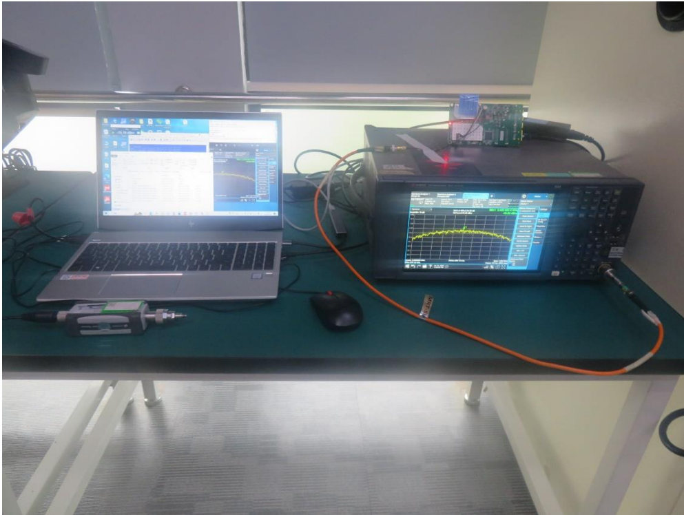
Description: Dynamic Frequency Selection Measurement Test Setup
