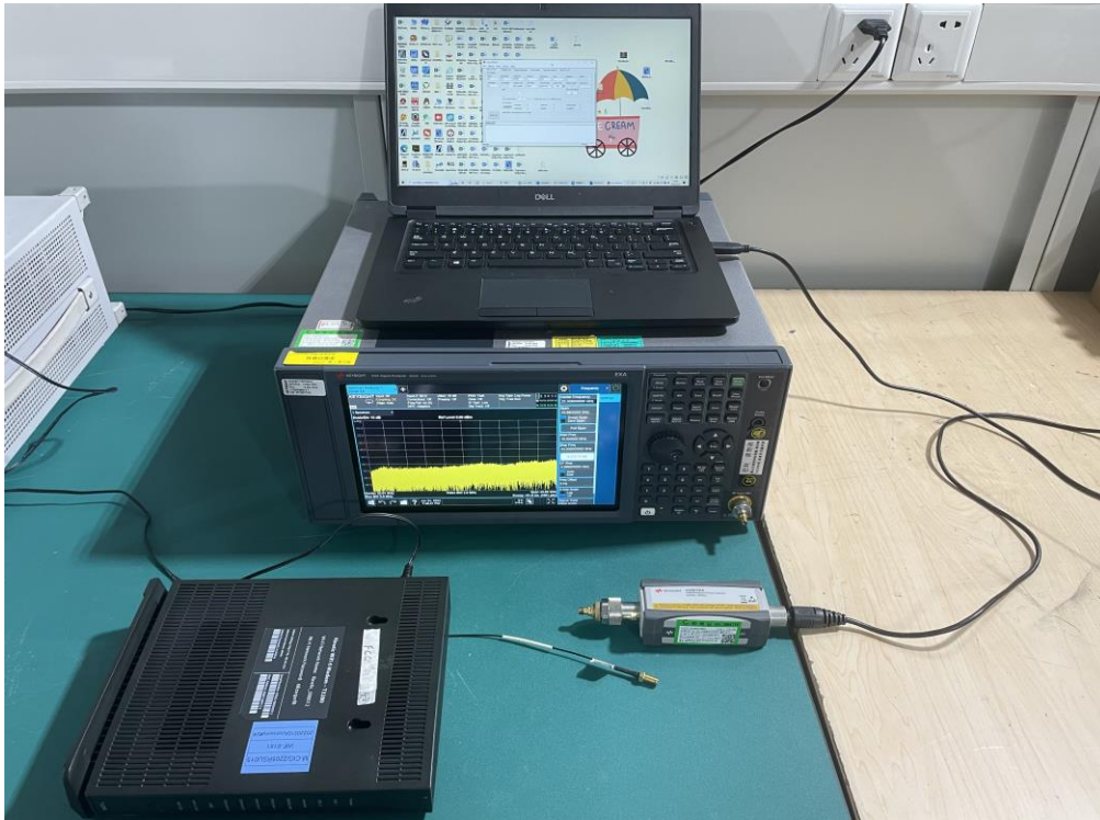
Description: Conducted Test Setup
