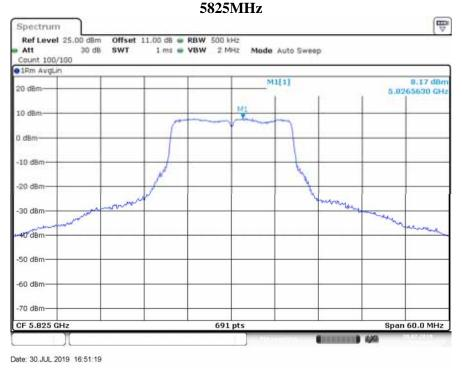
IEEE 802.11ac VHT20 Mode / 5725 ~ 5850MHz (chain 0) 5745MHz
