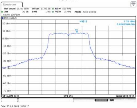
IEEE 802.11ac VHT20 Mode / 5725 ~ 5850MHz (chain 2) 5745MHz
