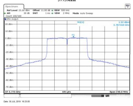
IEEE 802.11ac VHT80 Mode / 5725 ~ 5850MHz (chain 1) 5775MHz
