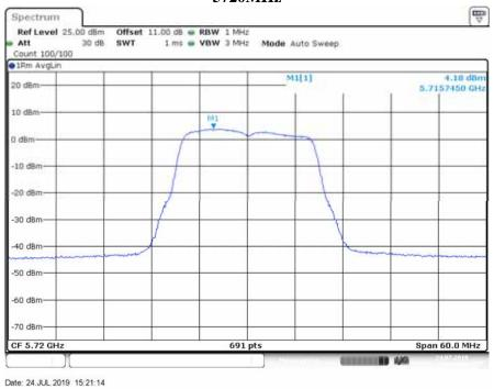
IEEE 802.11ac VHT20 Mode / 5470 ~ 5725MHz (chain 0) 5500MHz
