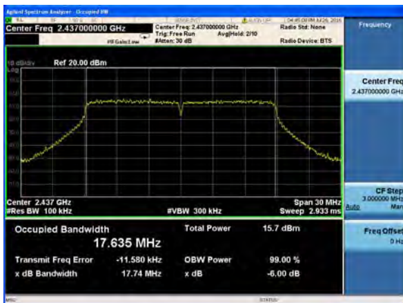
(802.11n20) 6dB Bandwidth plot on channel 6
