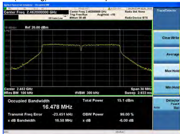
(802.11g) 6dB Bandwidth plot on channel 11
