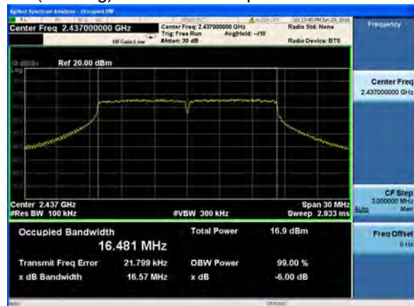
(802.11g) 6dB Bandwidth plot on channel 6
