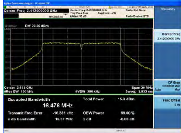
(802.11g) 6dB Bandwidth plot on channel 1
