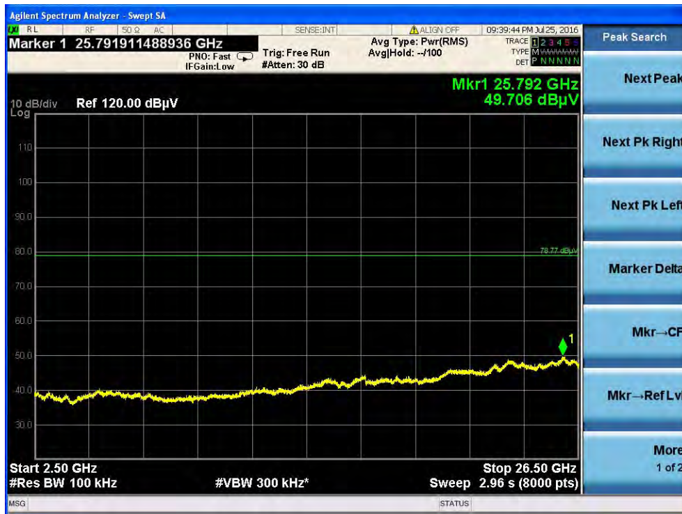
(802.11b) Emission not in Restricted Band plot on channel 11 Reference Level
