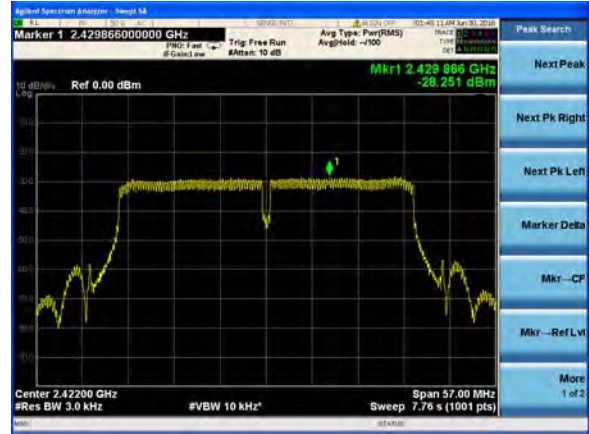
(802.11n40) PSD plot on channel 3
