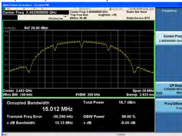
(802.11b) 6dB Bandwidth plot on channel 11
