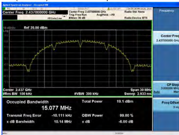
(802.11b) 6dB Bandwidth plot on channel 6
