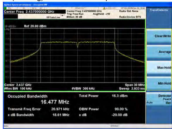
(802.11g) -20dB Bandwidth plot on channel 6
