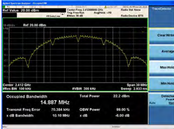
(802.11b) 6dB Bandwidth plot on channel 1
