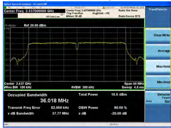
(802.11n40) -20dB Bandwidth plot on channel 6
