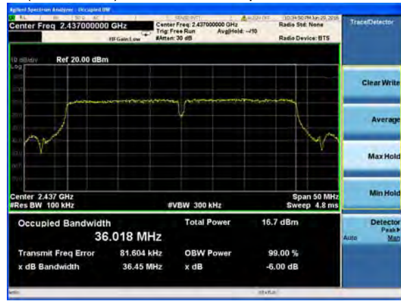
(802.11n40) 6dB Bandwidth plot on channel 6
