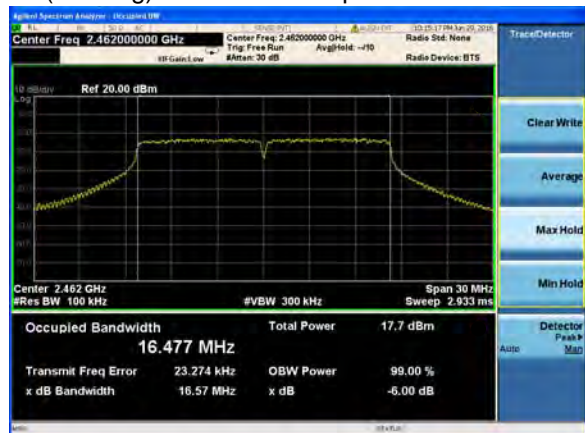
(802.11g) 6dB Bandwidth plot on channel 11
