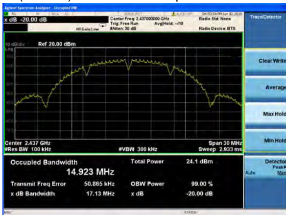
(802.11b) -20dB Bandwidth plot on channel 6
