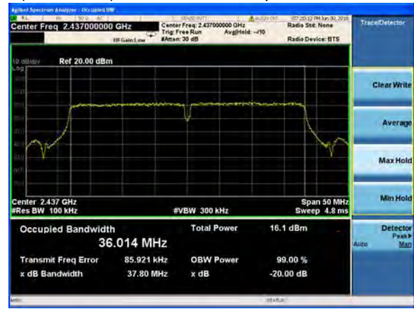
(802.11n40) -20dB Bandwidth plot on channel 6
