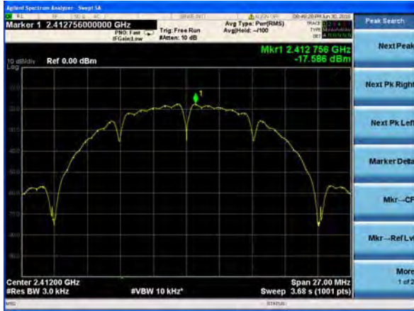
(802.11b) PSD plot on channel 1
