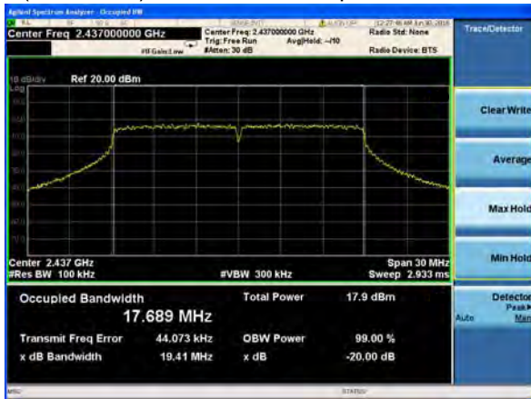
(802.11n20) -20dB Bandwidth plot on channel 6
