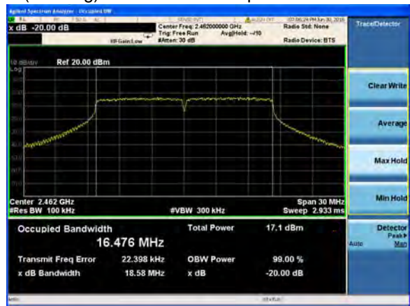
(802.11g) -20dB Bandwidth plot on channel 11
