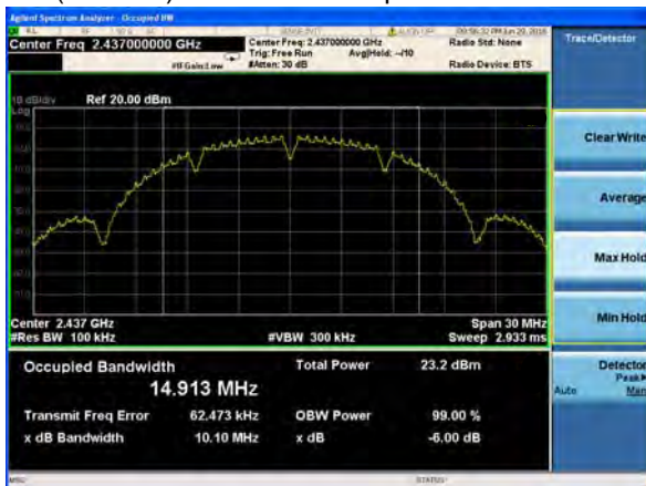
(802.11b) 6dB Bandwidth plot on channel 6
