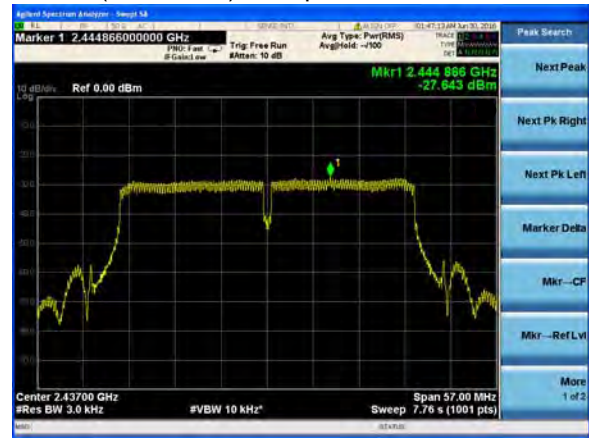
(802.11n40) PSD plot on channel 6
