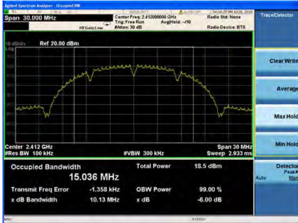
(802.11b) 6dB Bandwidth plot on channel 1
