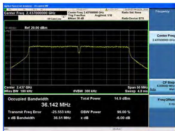
(802.11n40) 6dB Bandwidth plot on channel 6
