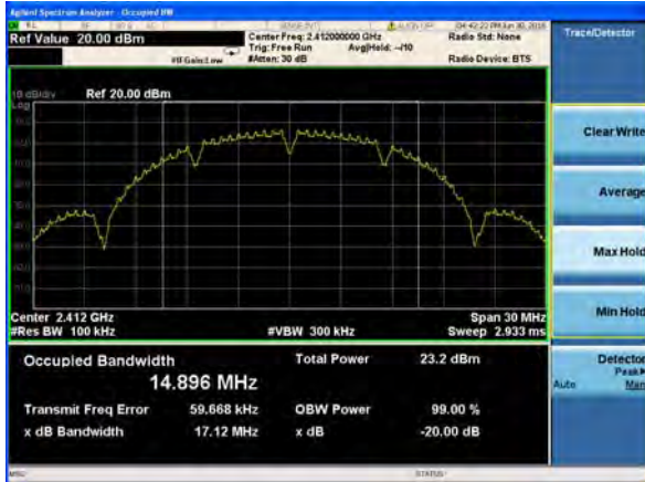
(802.11b) -20dB Bandwidth plot on channel 1
