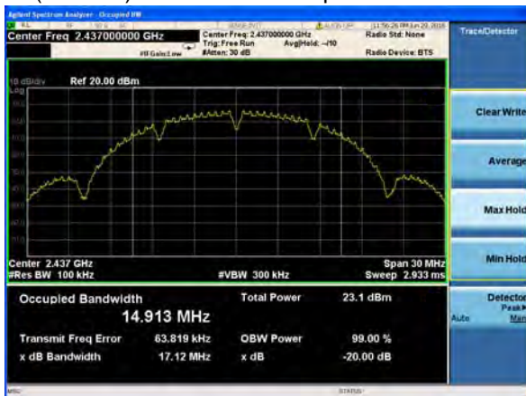
(802.11b) -20dB Bandwidth plot on channel 6
