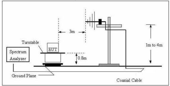
(C) Radiated Emission Test-Up Frequency Above 1GHz
