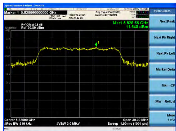
(802.11ac20) PSD plot on channel 165
