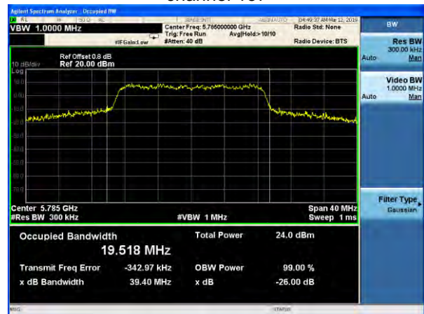
(802.11 n20) -26dB&99%Bandwidth plot on channel 157
