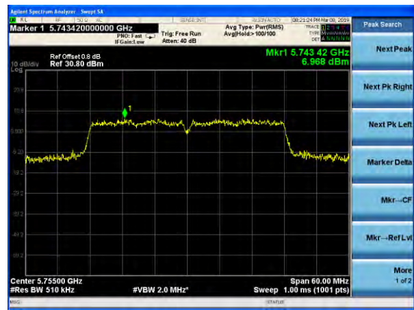
(802.11n40) PSD plot on channel 151
