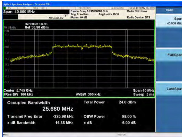
(802.11a) 6dB Bandwidth plot on channel 149
