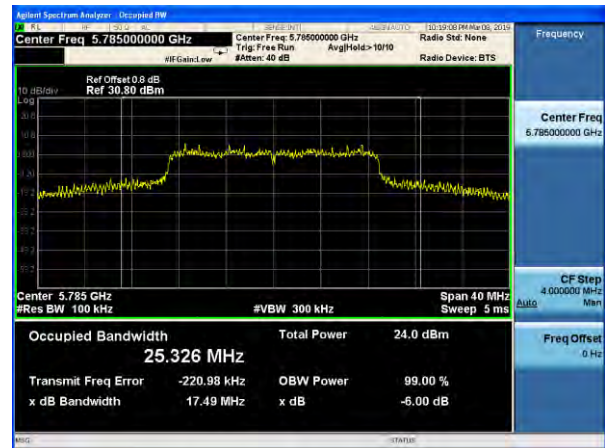
(802.11 AC20) 6dB Bandwidth plot on channel 157
