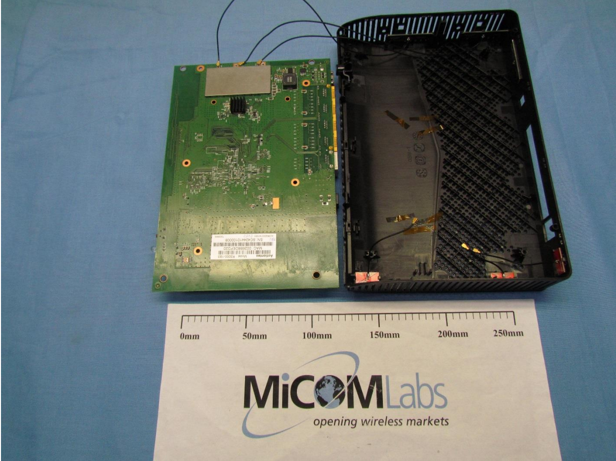
EUT back with 2.4GHz radio card connected to antenna
