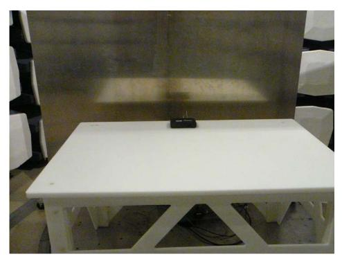
14.2 AC Line Conducted Emission – Side View
