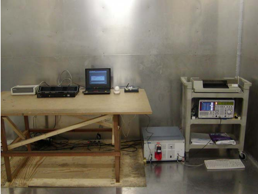
Conducted Emission - Front View
