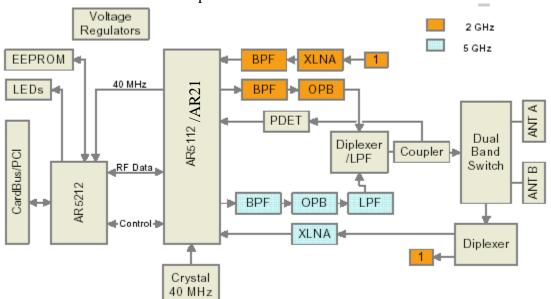
The AR5212 is the origin and destination for all the front-end signals. Both transmit (Tx) and receive (Rx) signals are transferred by the AR5112 to either a 5GHz front-end, or a 2.4GHz front end.
