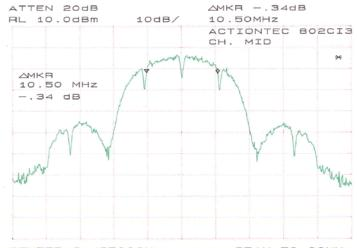
CENTER 2.43700GHz SPAN 50.00MHz \*RBW 100kHz \*VBW 100kHz \*SWP 50.0ms
