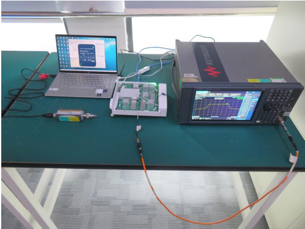
Description: DFS Test Setup – Master
