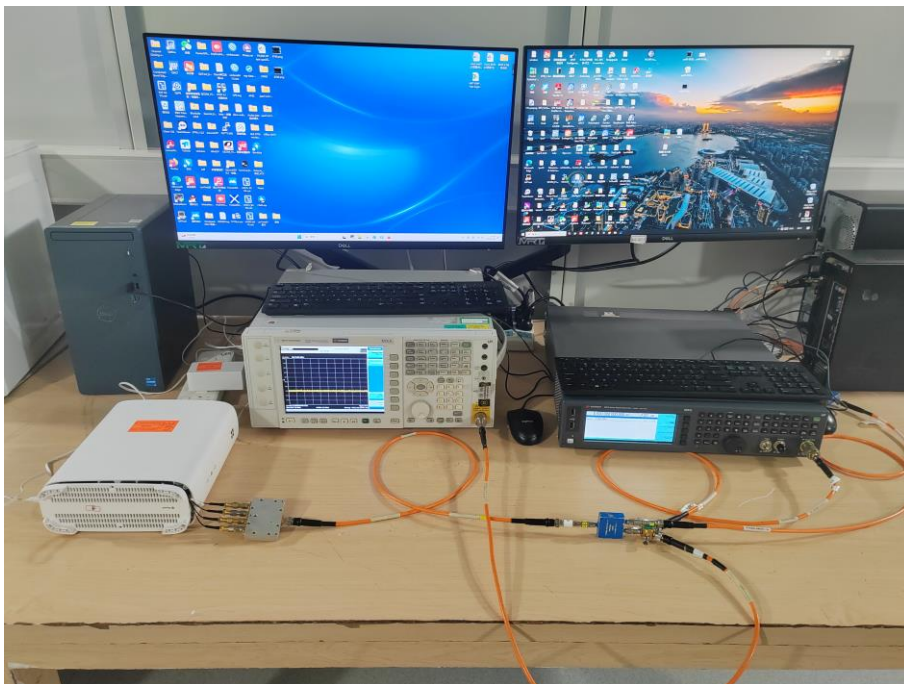
Description: DFS Conducted Test Setup
