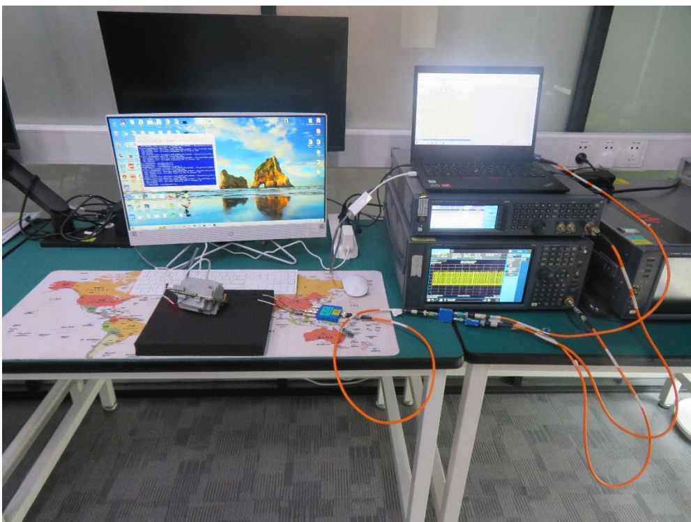
Description: Dynamic Frequency Selection Measurement Test Setup
