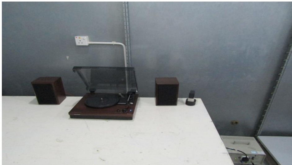
Measurement of Conducted Emission Test Set Up
