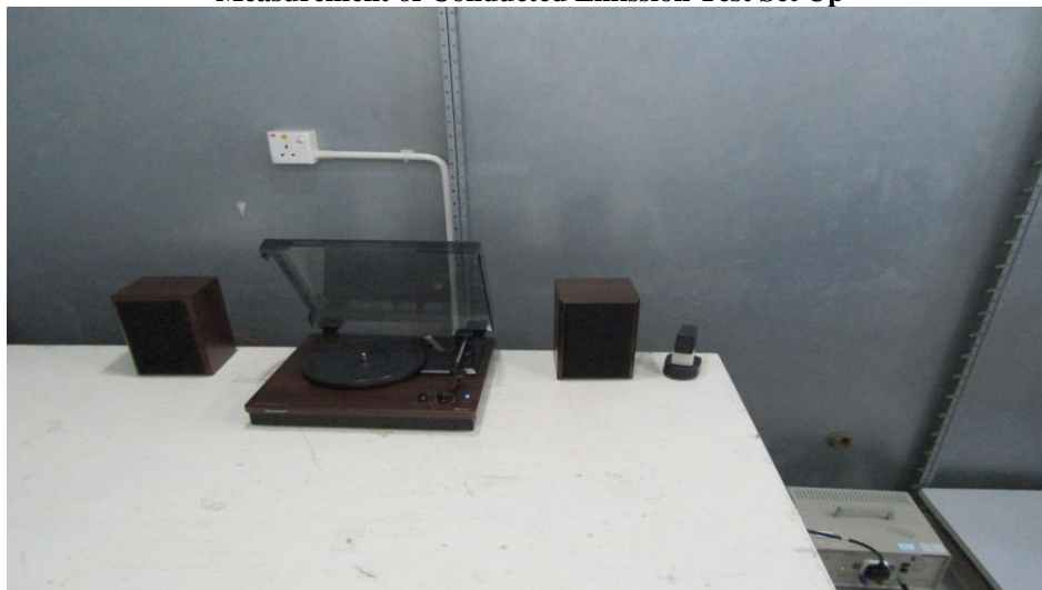
Measurement of Conducted Emission Test Set Up
