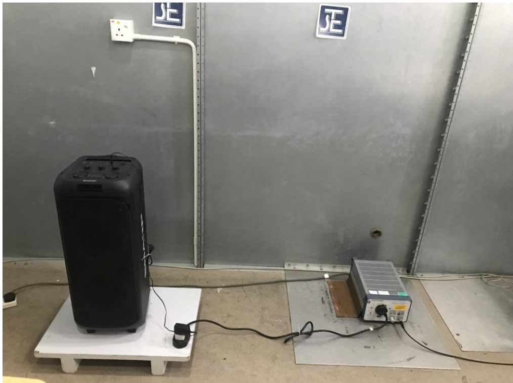
Measurement of Conducted Emission Test Set Up
