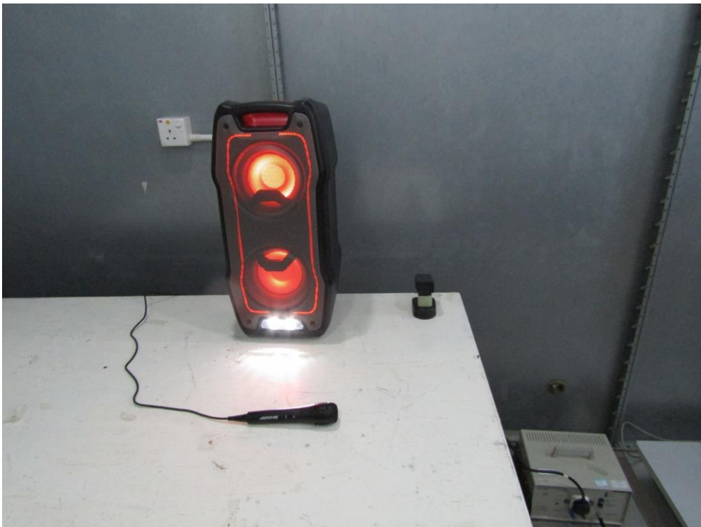
Measurement of Conducted Emission Test Set Up
