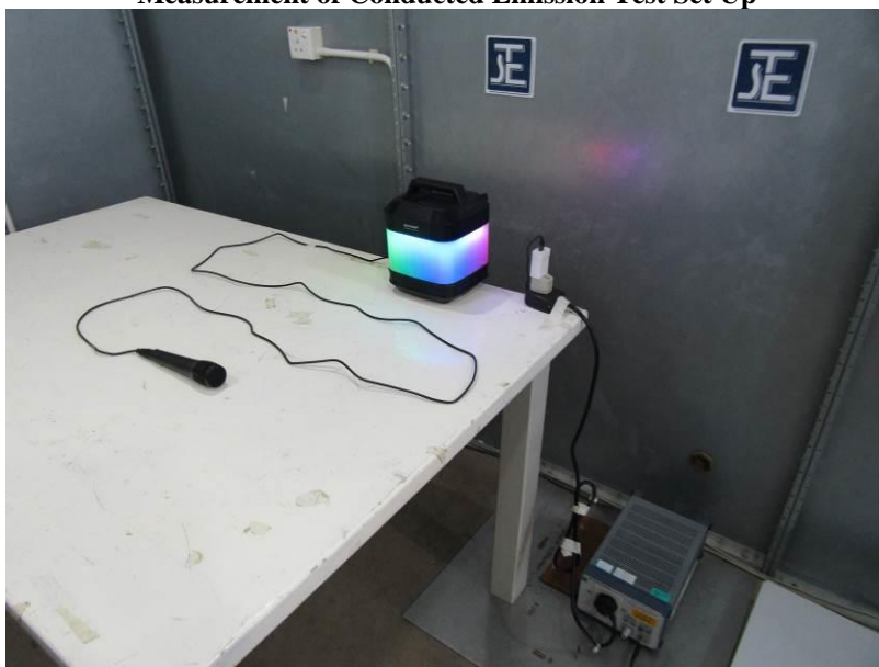
Measurement of Conducted Emission Test Set Up
