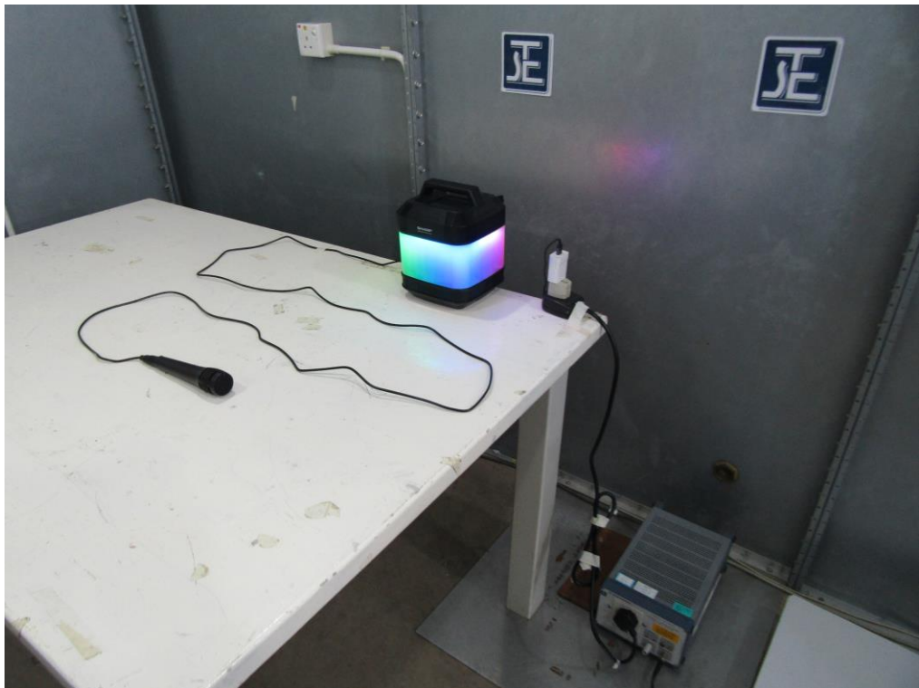
Measurement of Conducted Emission Test Set Up
