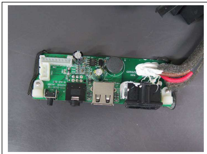
Internal Configuration 11 (Connector board)
