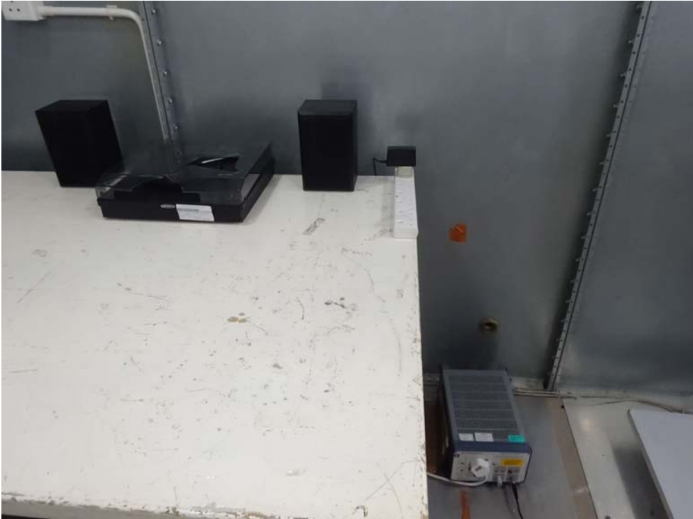
Measurement of Conducted Emission Test Set Up
