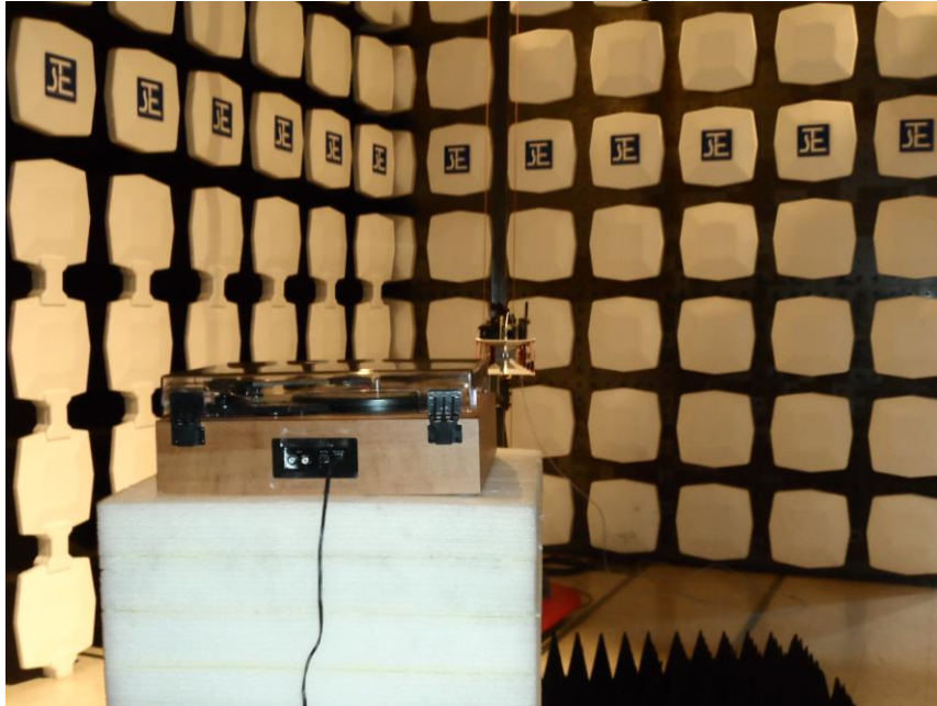
Measurement of Conducted Emission Test Set Up
