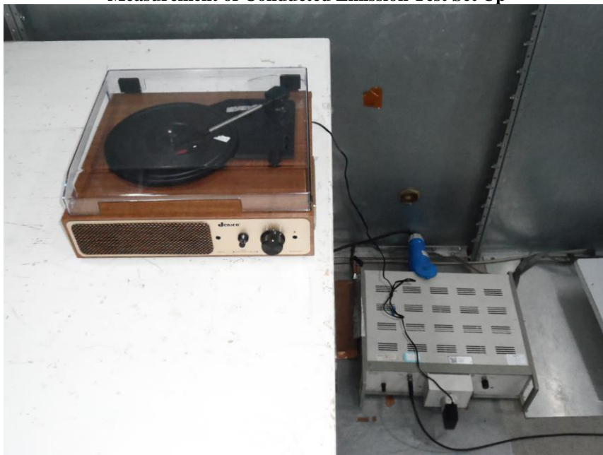
Measurement of Conducted Emission Test Set Up
