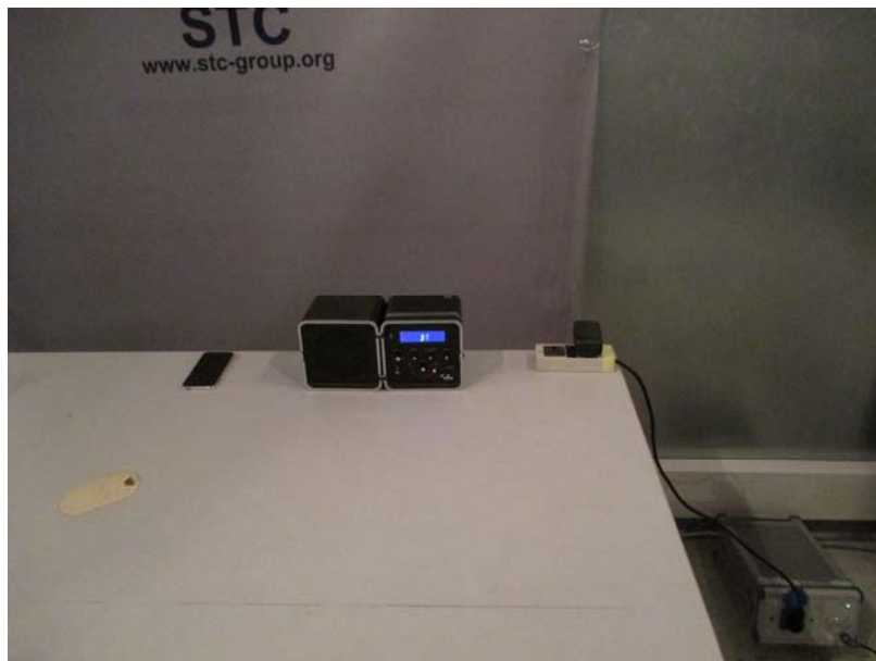
Measurement of Conducted Emission Test Set Up
