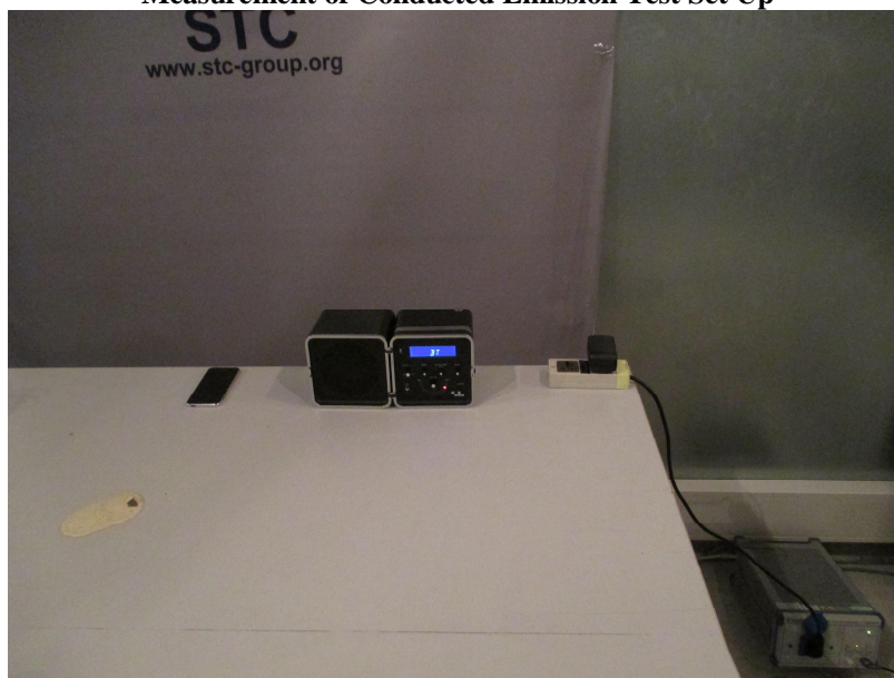
Measurement of Conducted Emission Test Set Up
