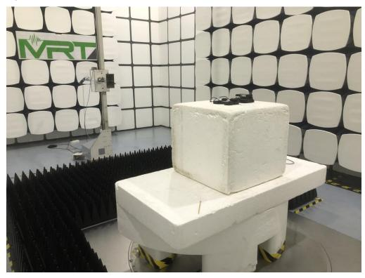
Description: Radiated Spurious Emission Test Setup for 18GHz - 26GHz
