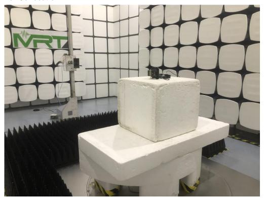
Description: Radiated Spurious Emission Test Setup for 18GHz - 26GHz
