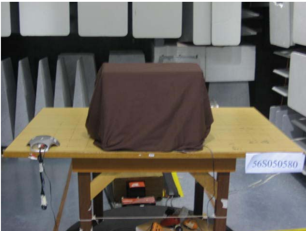
Radiated Emissions Setup (Rear View)
