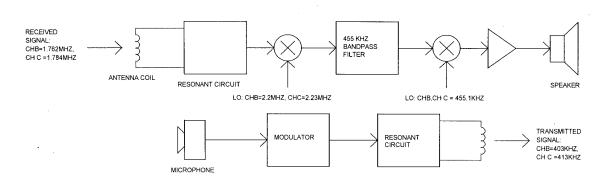
For the receiving parts, the antenna coil receives the signal (1.762MHz / 1.784MHz) from the base. The received signal is then mixed with the LO (2.2MHz / 2.23MHz) and pass through a 455kHz band-pass filter. The resulting signal from the filter will mixed with the second LO (455.1kHz) to give the voice signal. The voice signal will be amplified and output to the speaker.
