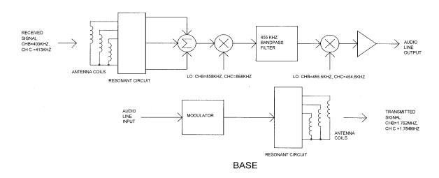
For the receiving parts, the antenna coils receives the signal (403kHz / 413kHz) from the headset and sum up together. The received signal is then mixed with the LO (858kHz / 868kHz) and pass through a 455kHz band-pass filter. The resulting signal from the filter will mixed with the second LO (455.5kHz / 454.6kHz) to give the voice signal. The voice signal will be amplified and output to the audio line input of the user cellular phone.
