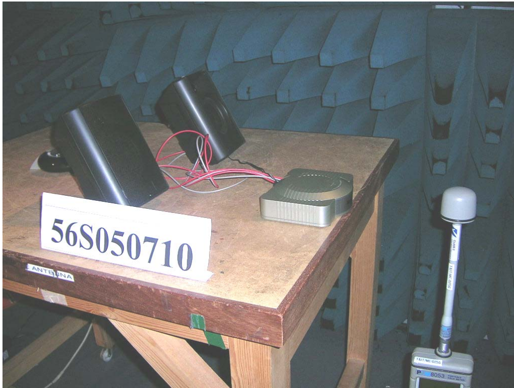
Maximum Permissible Exposure (MPE) Test Setup
