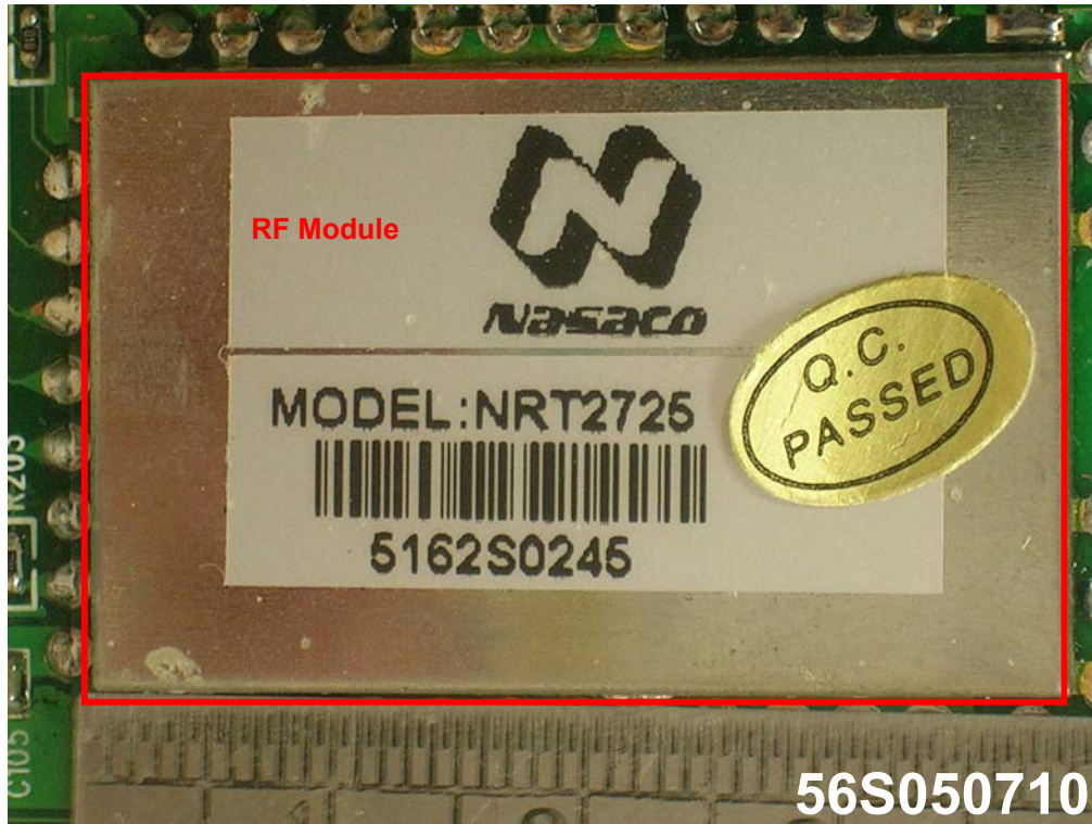
RF Module Circuit with RF Shield
