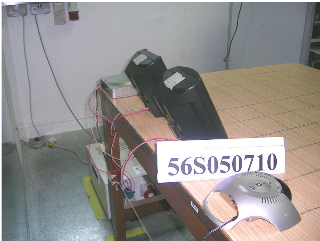
Conducted Emissions Test Setup (Rear View)
