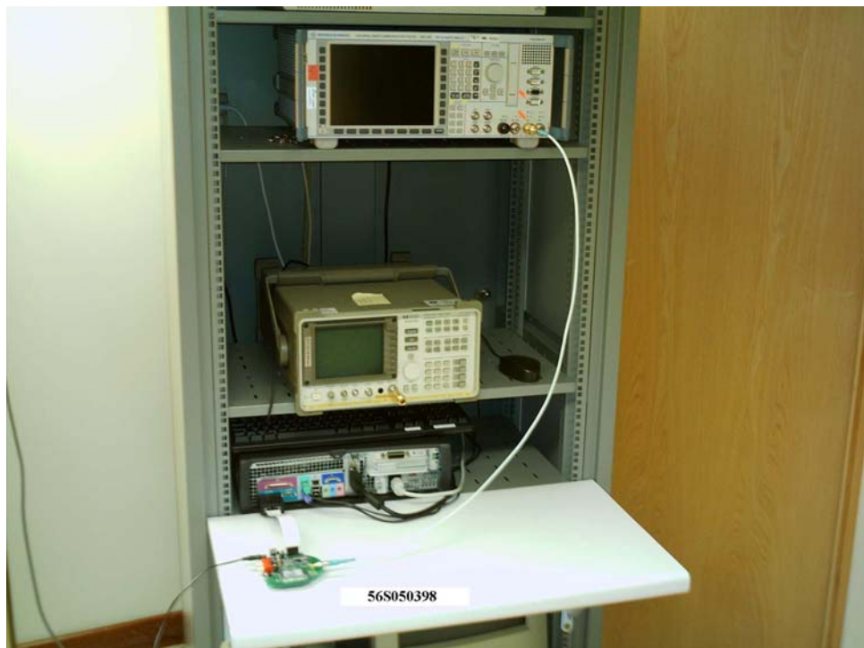
Maximum Peak Power Measurement Test Setup
