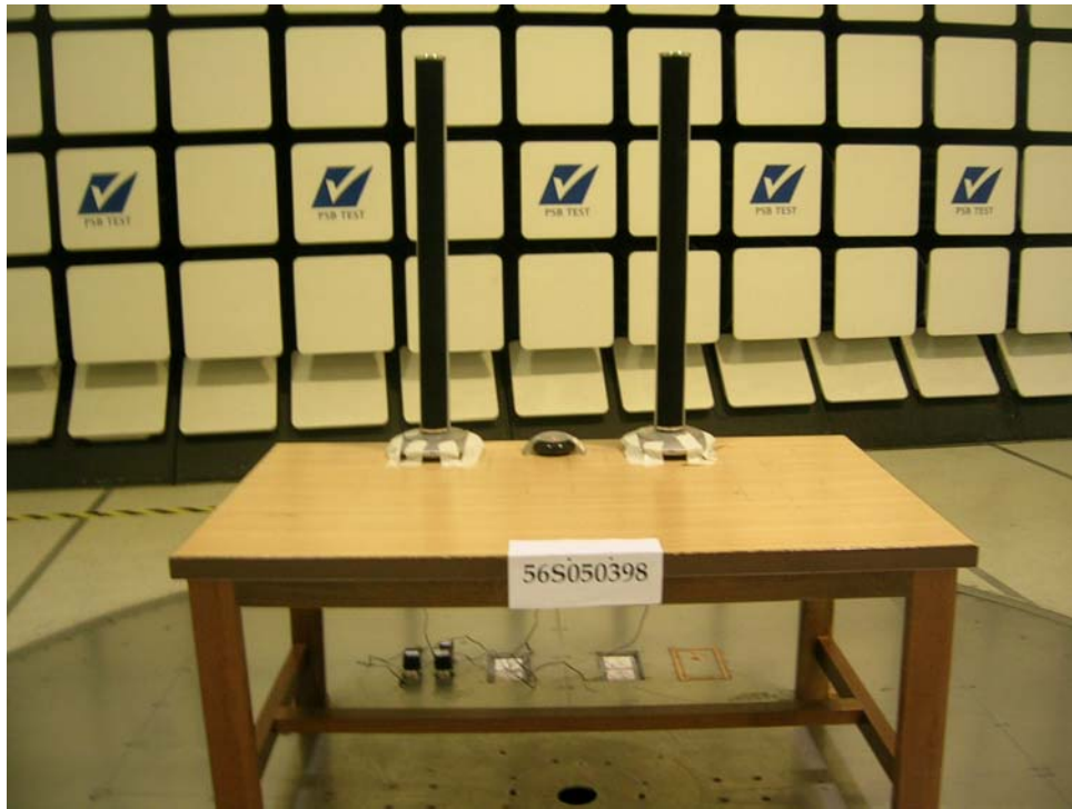
Radiated Emissions Setup (Front View)
