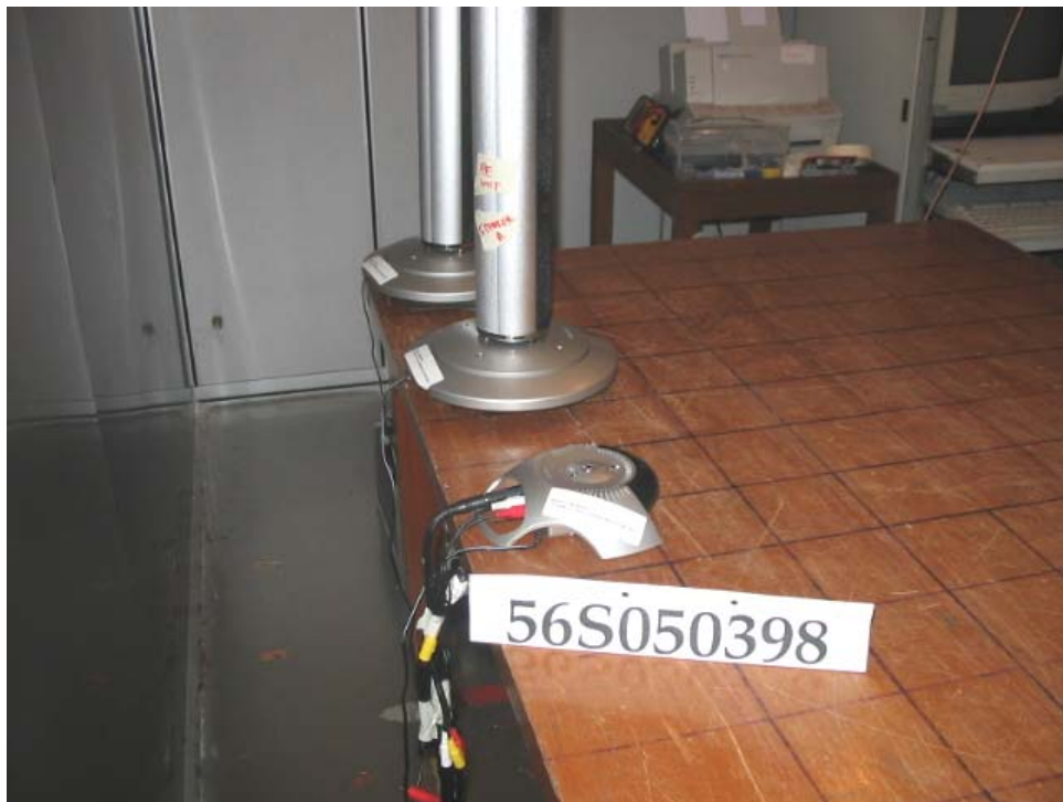
Conducted Emissions Setup (Rear View)
