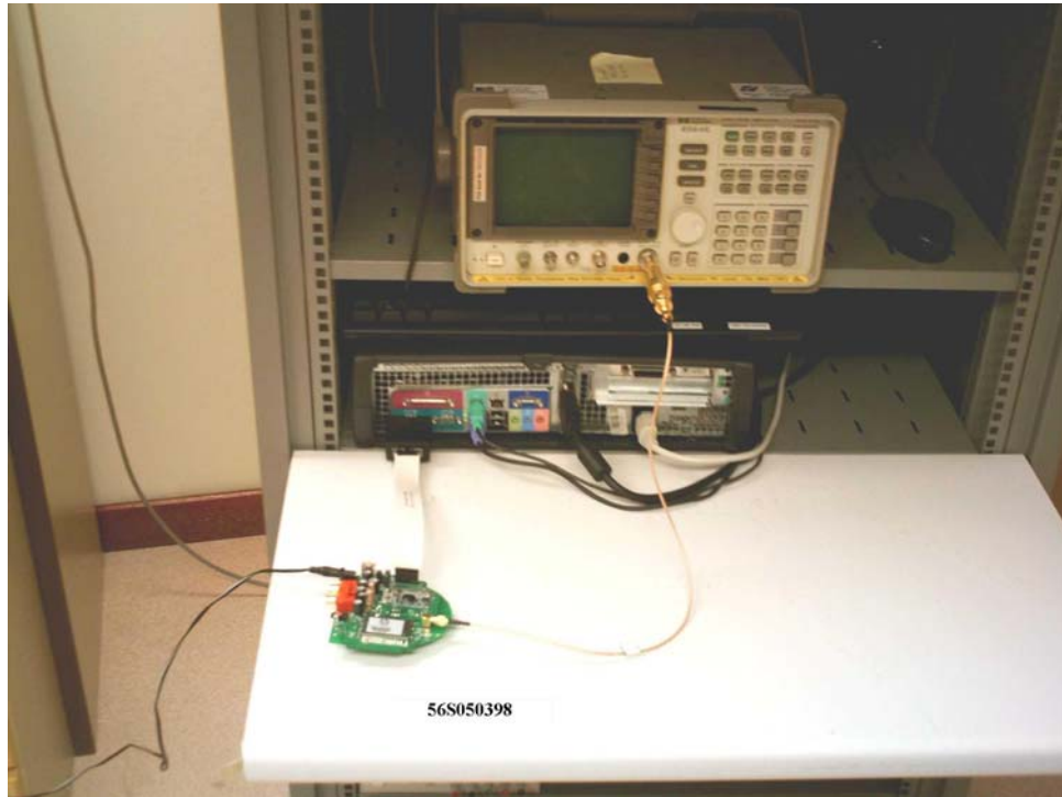
Carrier Frequency Separation Measurement Test Setup
