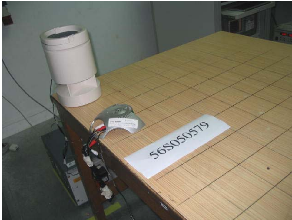
Conducted Emissions Setup (Rear View)
