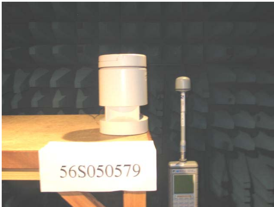
Maximum Permissible Exposure Measurement Test Setup
