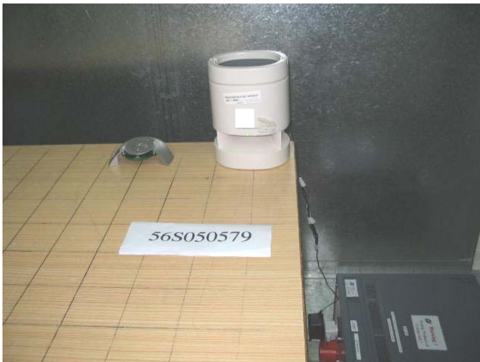
Conducted Emissions Setup (Front View)
