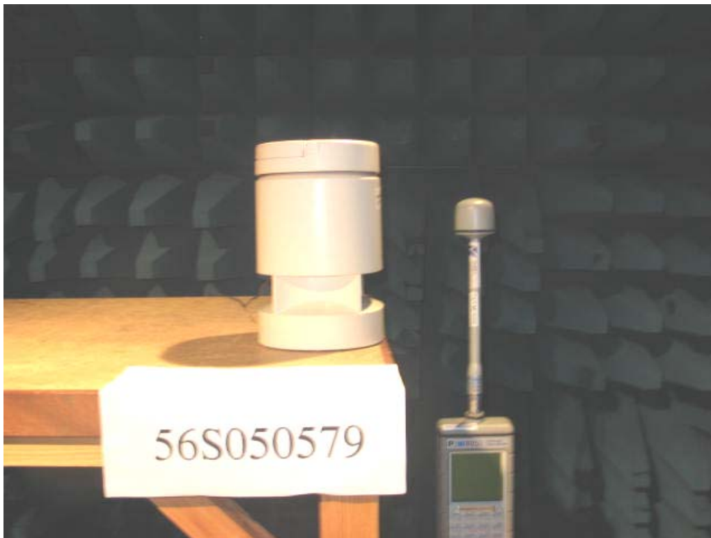
Maximum Permissible Exposure Measurement Test Setup
