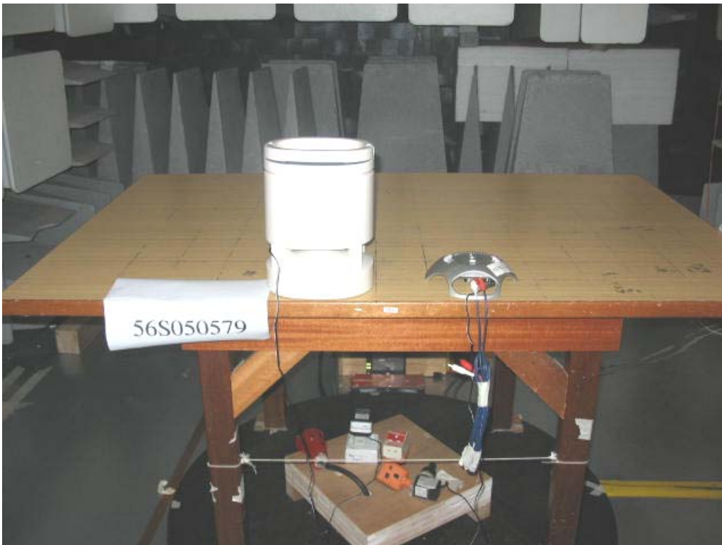
Radiated Emissions Setup (Rear View)
