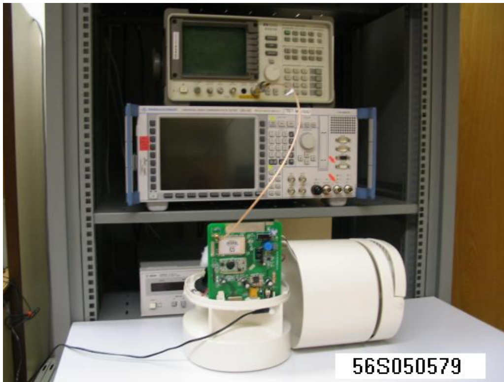
Spectrum Bandwidth Measurement Test Setup
