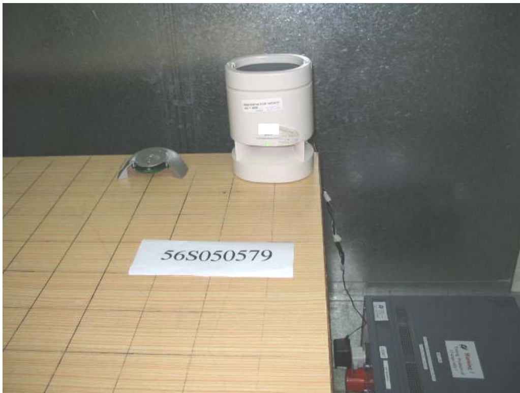
Conducted Emissions Setup (Front View)
