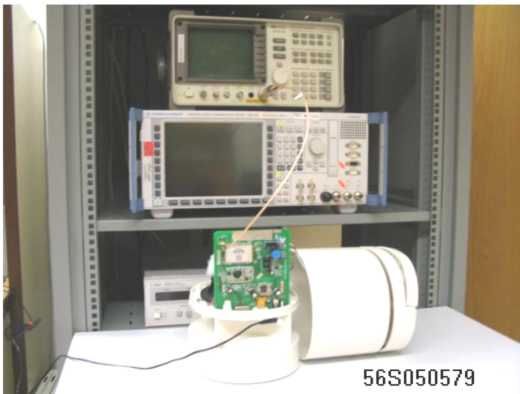
Number of Hopping Frequencies Measurement Test Setup
