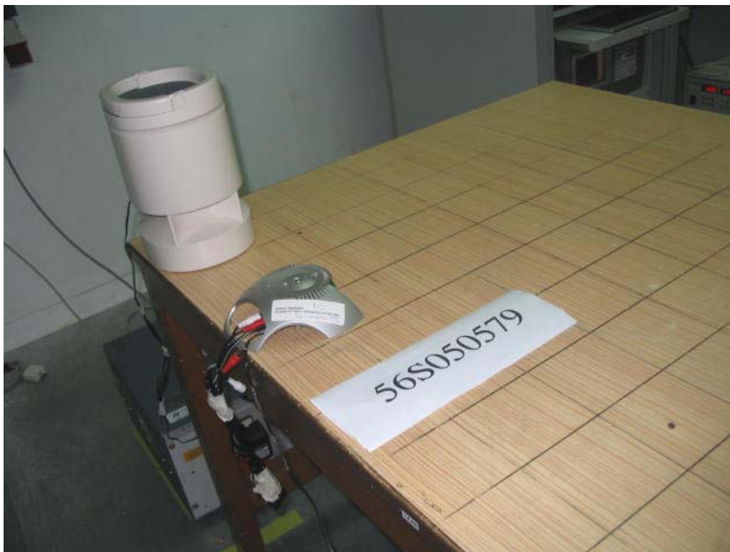
Conducted Emissions Setup (Rear View)
