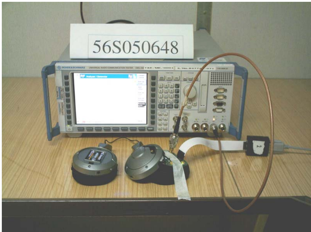
Conducted Power Measurement Setup
