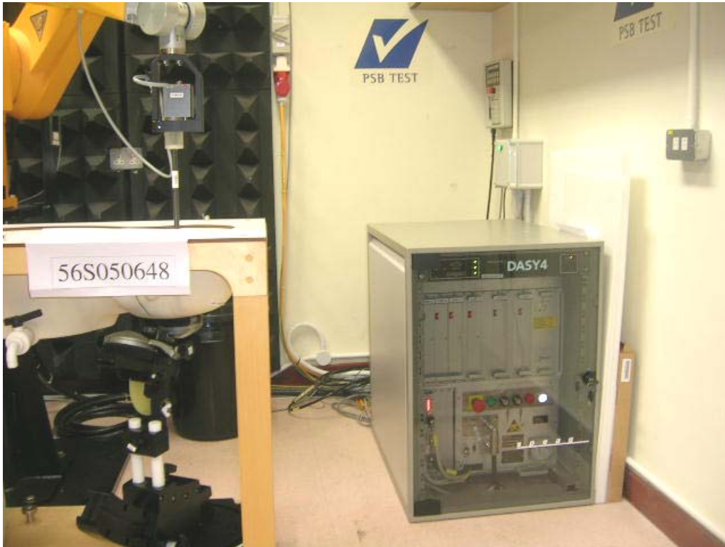
SAR Test Setup (Device at Head Phantom)
