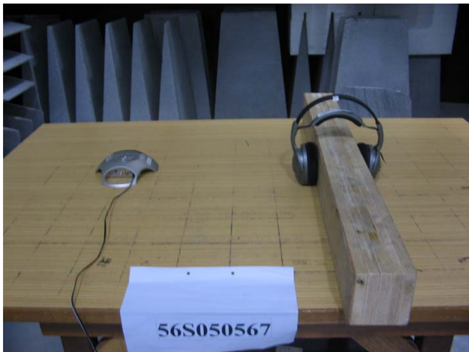
Radiated Emissions Setup (Rear View)
