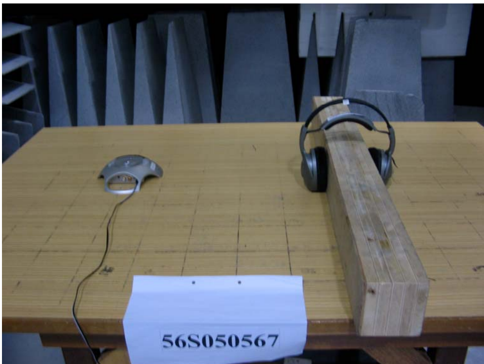
Radiated Emissions Setup (Rear View)
