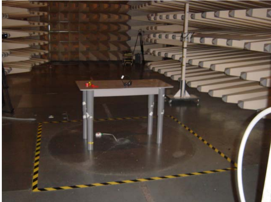
Set-up for Radiation Emission (Transceiver)
