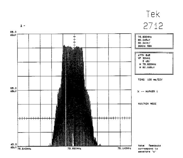
Result : The field strength of any emission within the operation band did not exceed 98  $dB(\mu V/m)$  for average value or 118  $dB(\mu V/m)$  for peak value. Refer to page 9 &12 for the recorded value for the emission at the fundamental frequency.
