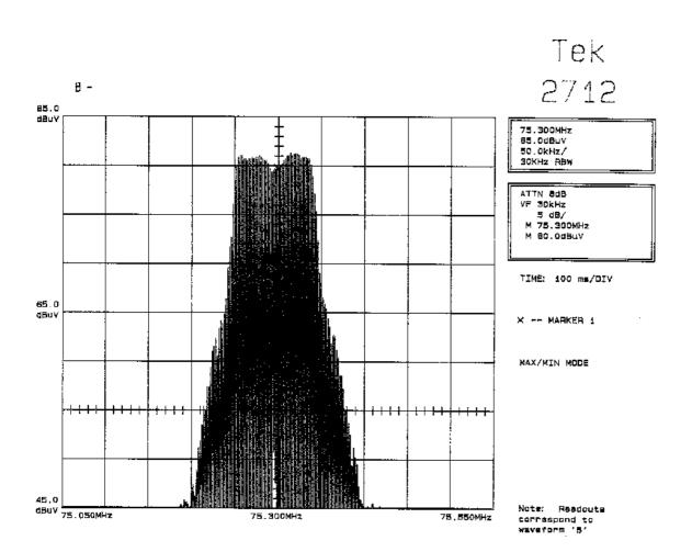
Result : The field strength of any emission within the operation band did not exceed 98  $dB(\mu V/m)$  for average value or 118  $dB(\mu V/m)$  for peak value. Refer to page 9 &12 for the recorded value for the emission at the fundamental frequency.
