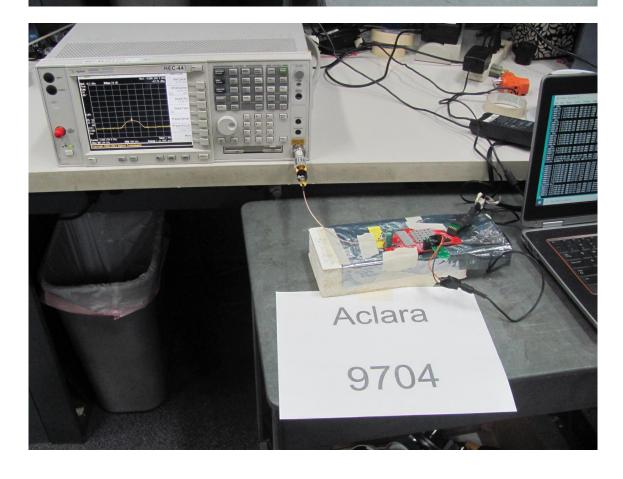
Photographs of Voltage and Temperature Stability Test Setup
