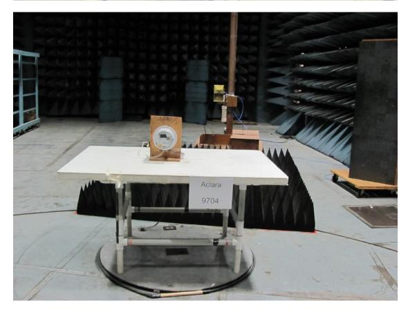
Photographs of Antenna Conducted Emissions Test Setup
