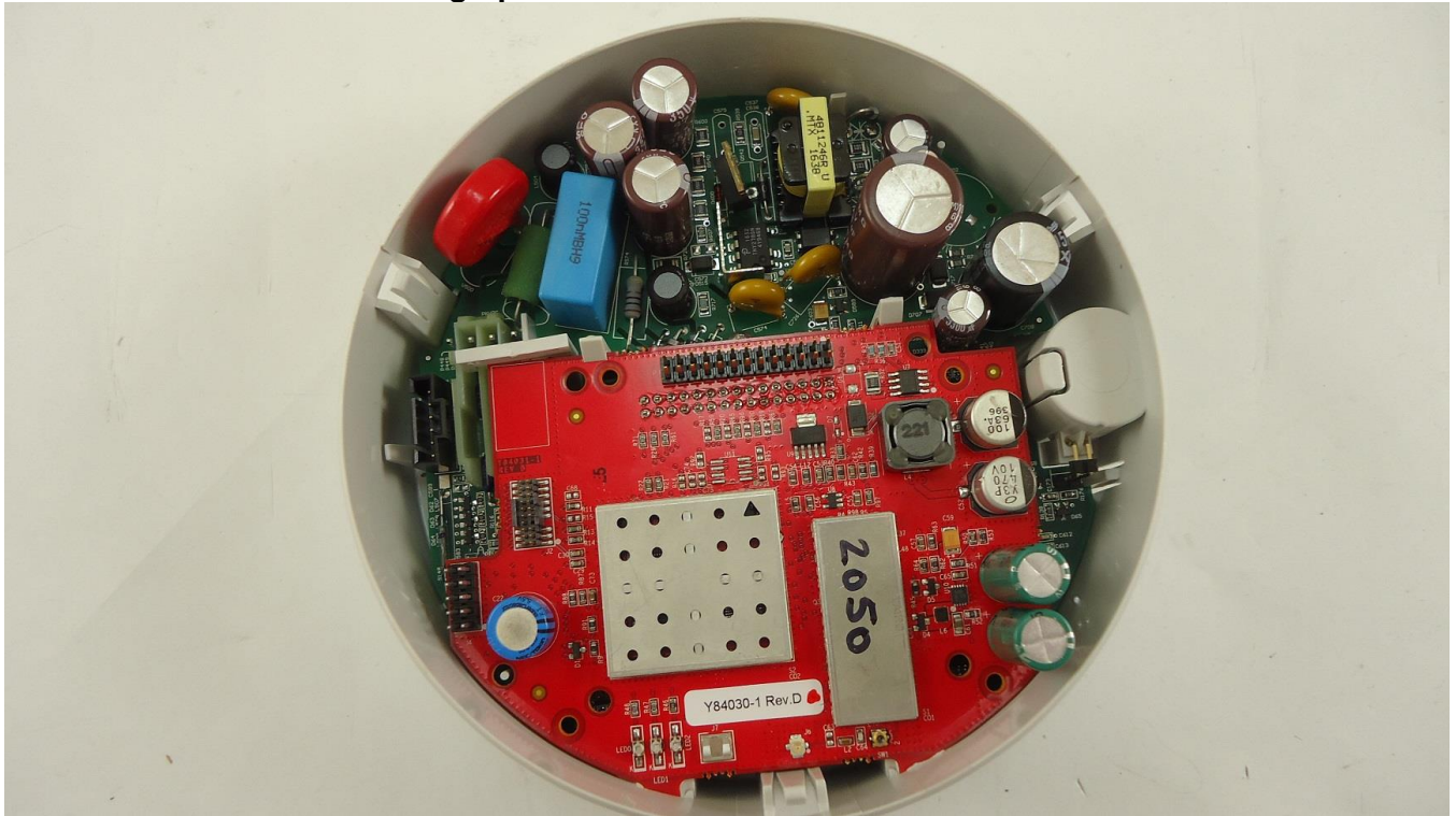
Photograph of RF Board Installed in Meter Board
