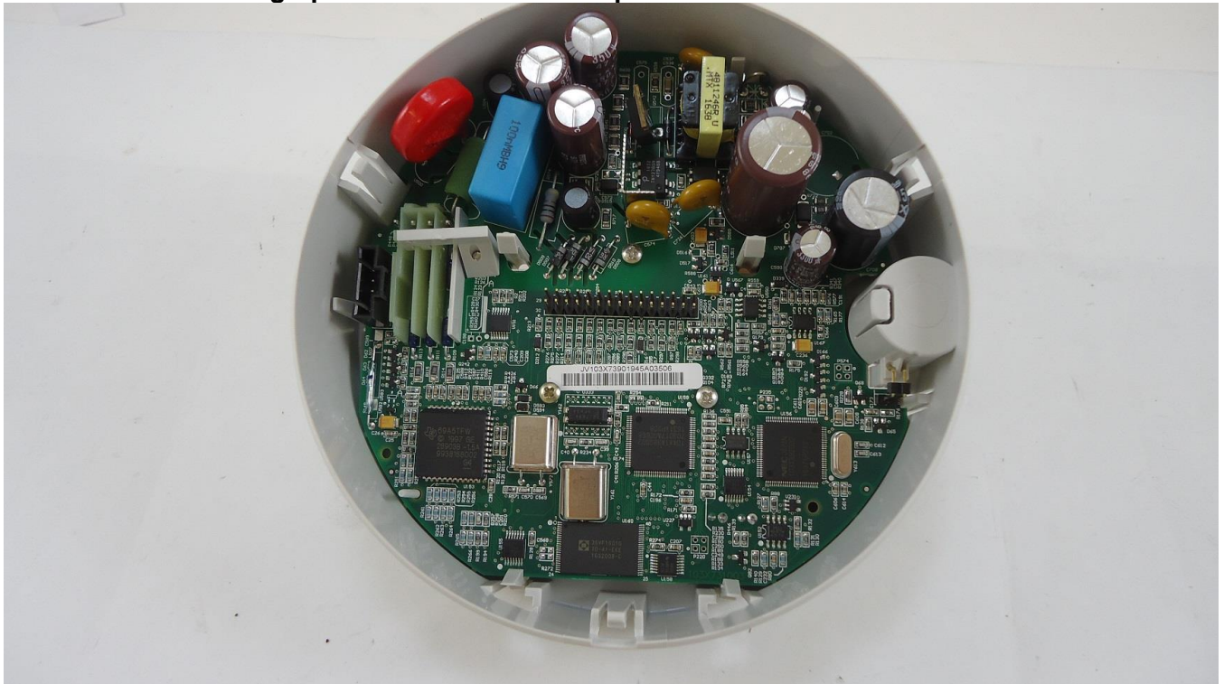
Photograph of Meter Board: Component side with shield removed
