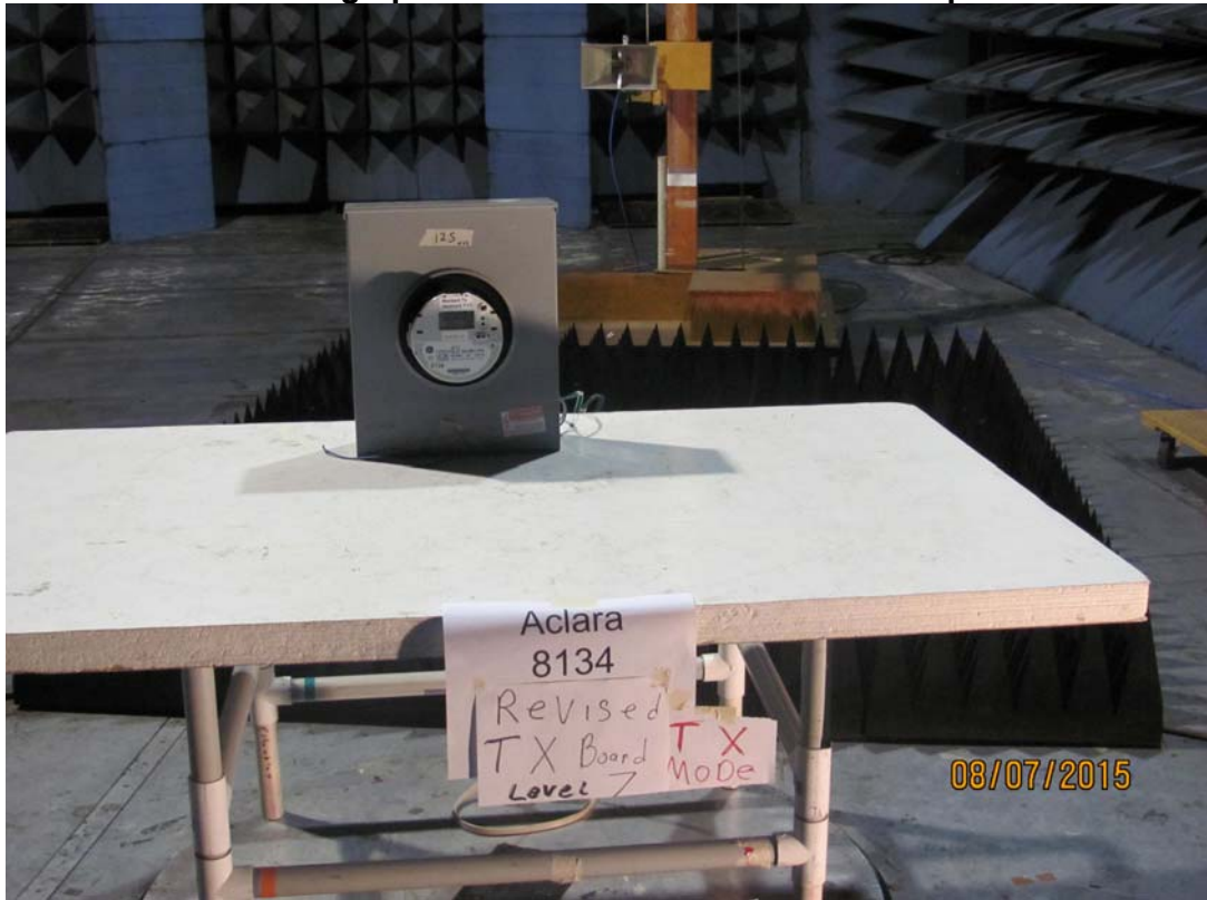
Photograph of Radiated Emissions Test Setup
